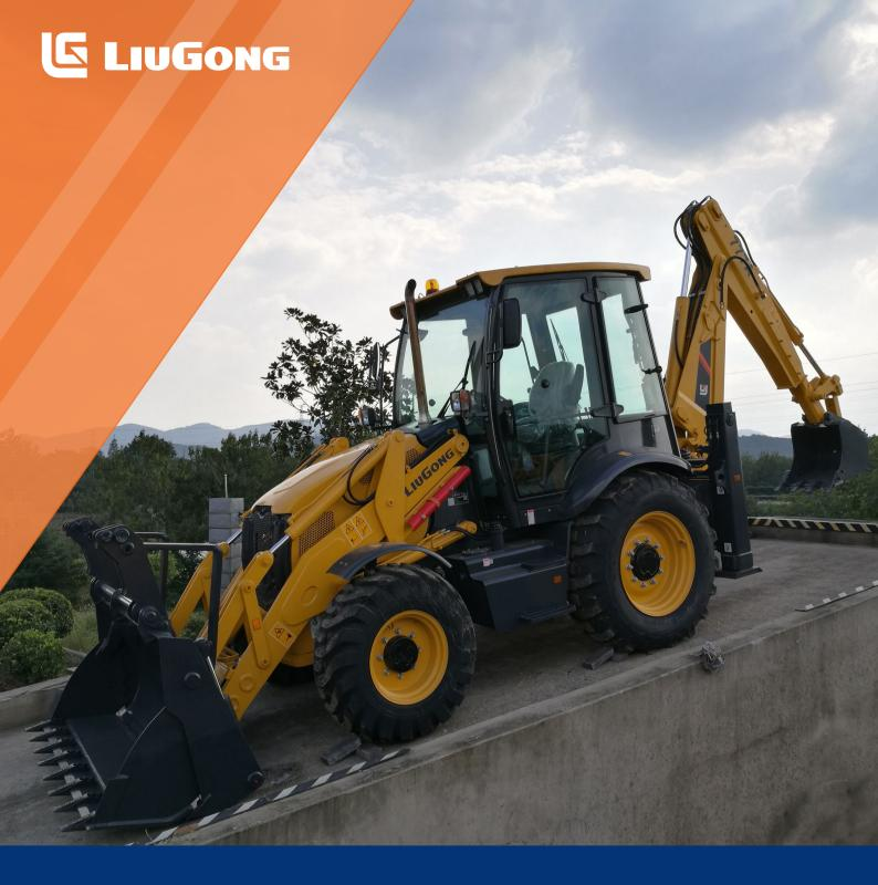
Engine Perkins 1104D-44TA Gross Power 74.5 kW (100 hp / 101 ps) @ 2,200 rpm Net Power 72 kW (97 hp / 98 ps ) @ 2,200 rpm Maximum Speed 36 km/h Standard Loader Bucket Capacity 1.0 m³ Standard Backhoe Bucket Capacity 0.2 m³ Operating Weight 8,400 kg
